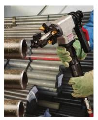
Bevel, face and bore simultaneously up to 4.5" (114.3mm) o.d.
