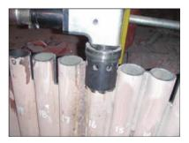
Membrane removal heads and Overlay removal heads efficiently remove material from between boiler tubes.
