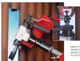
Ideal for limited access areas, the "Wart" MILLHOG® requires a minimum width of 2-5/8" clearance to fit between tubes, and easily clamps into place with the Knurled Knob and Heavy Duty Ratchet.
