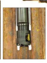
The Standard Ground is only 1.5in wide and is ideal for end prepping all boiler tube materials and accessing single tubes in a boiler tube waterwall. It can also be equipped with a membrane removal head for removing membrane from boiler tubes.
